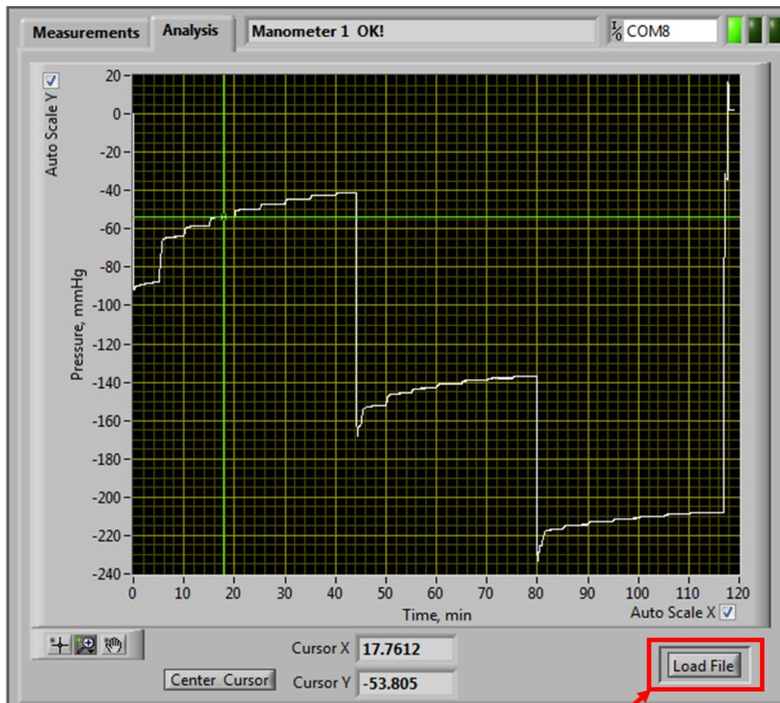
**Fig. 18 The window for saved data analysis (Analysis tab)
