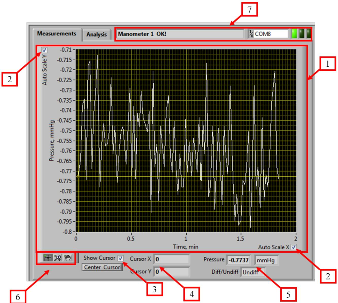
**Figure 15. The window for the measurement of current value of pressure by first manometer. “Measurements” Tab.**
