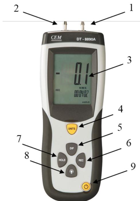
**Fig. 10. Differential manometer**
